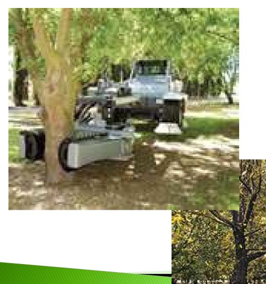
A Shaker is used to get the nuts off of the Trees
